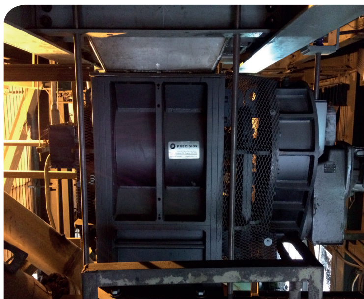
Precision PMDS-18 Self-Cleaning Rotary Valve installed at Lehigh Northeast Cement in Glens Falls, NY.
